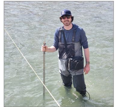
Below: Jonah Howe collects depth and velocity measurements in the river.
