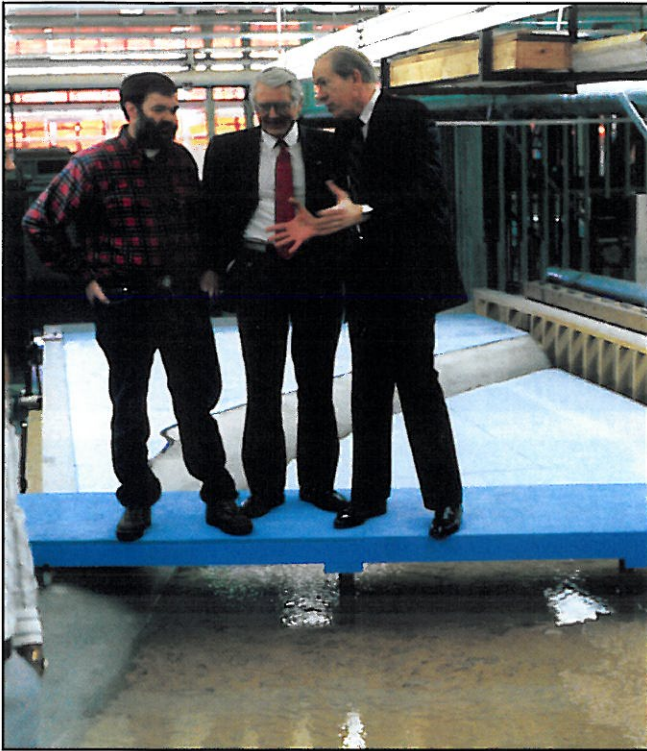
Engineers view and discuss a Bureau of Reclamation model of the South Platte River through Englewood that was built to test hydraulics.
